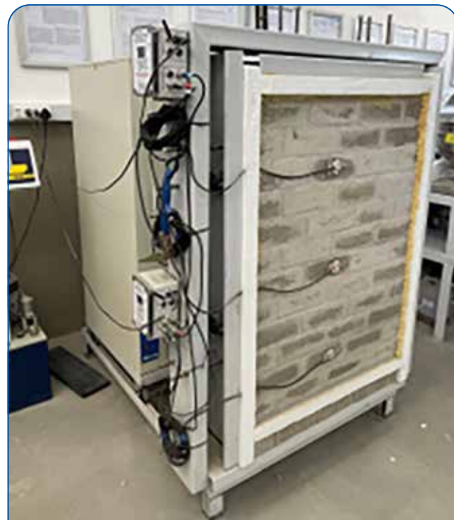
Full-scale thermal property testing unit designed and fabricated in the Green Concrete Lab
