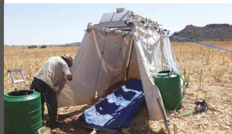
A portable rainfall simulator used to measure runoff and soil erosion rates on different landuse/soil combinations near Ladybrand
